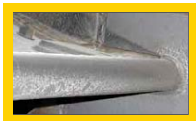
Fan blade protected with Conforma Clad liner.
