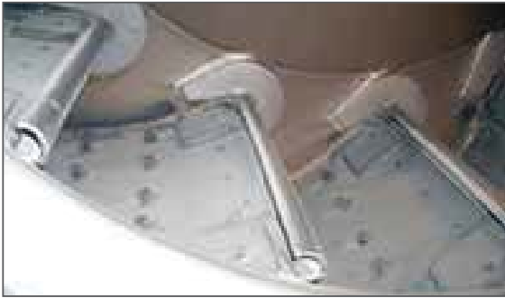
Leading edge and center plate protection.
