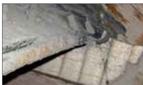
Fan blade protected with chrome carbide weld overlay liner.
